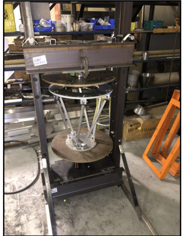
Compression tester fit test for hexapod thrust structure compression testing
