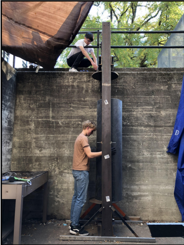
Compression testing setup for testing 18" diameter, 72" tall carbon fiber bodytube
