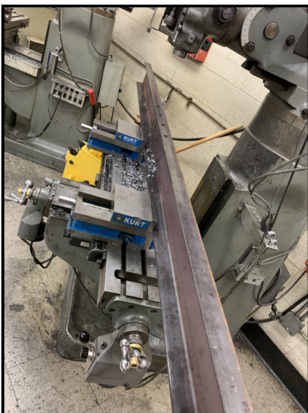
Manual Machining setup for dowel pin holes
