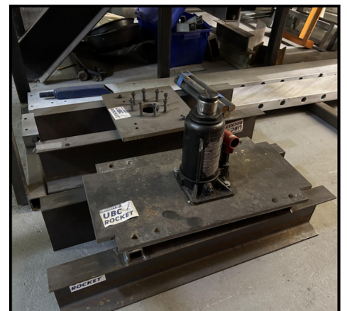
Assembled compression tester C-channel cross-beams (2x) with hydraulic jack (bottom) and load cell mount (top)
